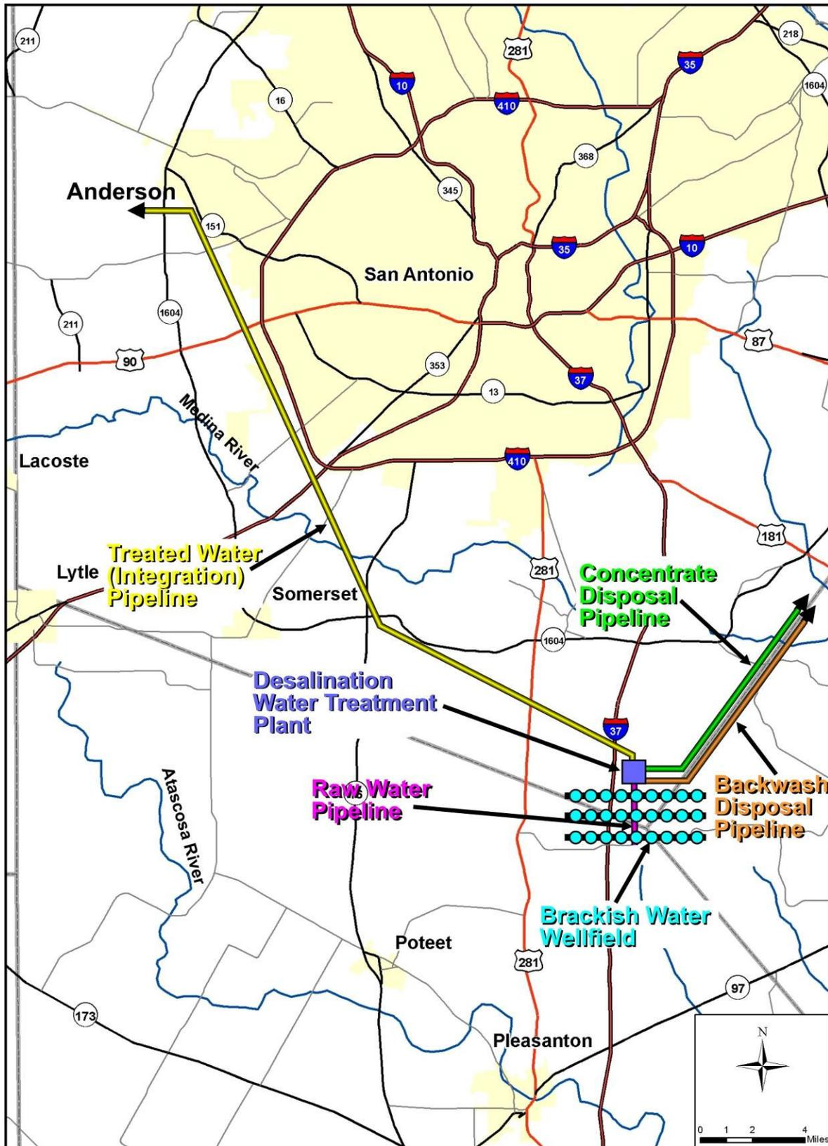
Figure 4-1. SAWS Local Wilcox Desalination Project
