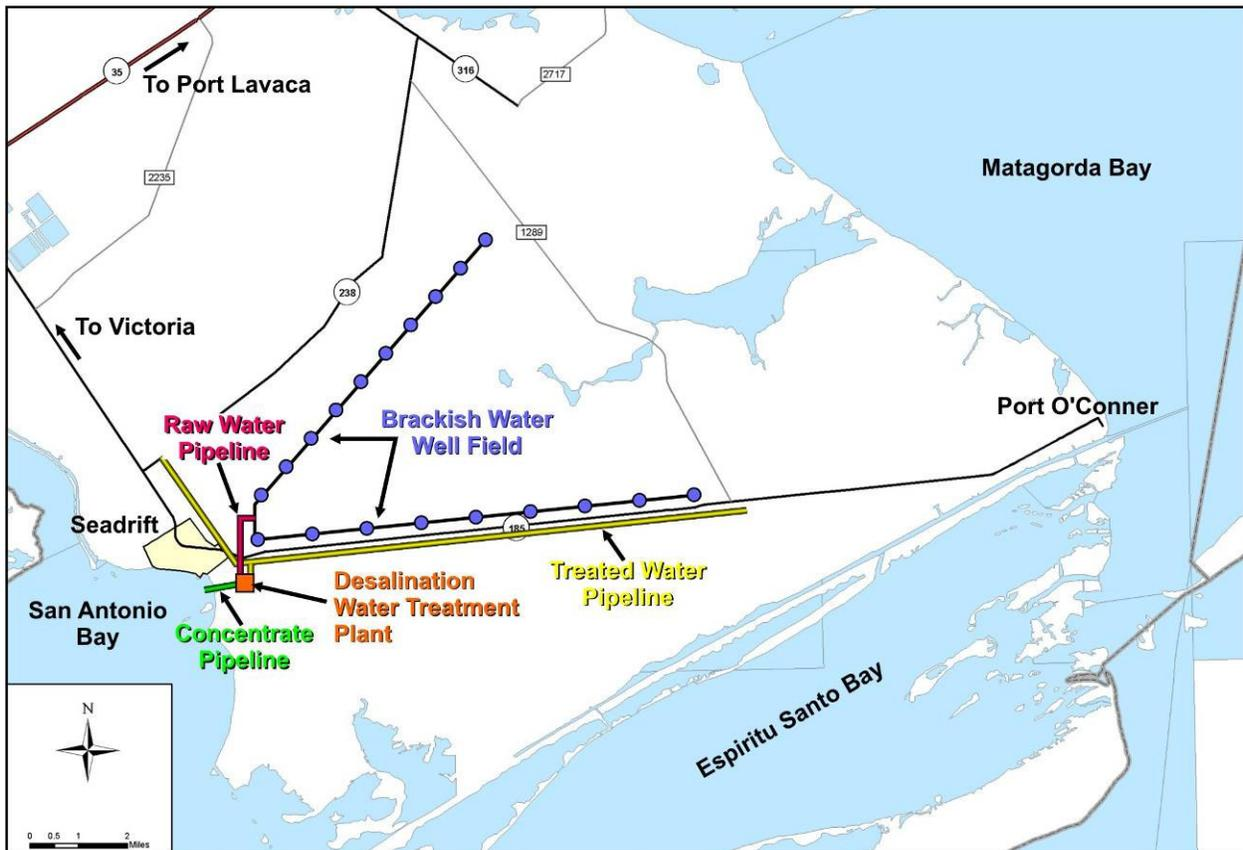
**Figure 2-1. Southern Calhoun County Brackish Groundwater Desalination Project**
