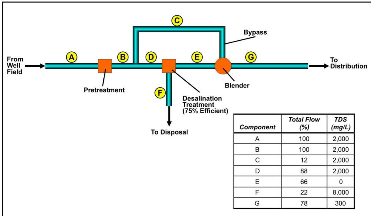
**Figure 2-2. Flow Diagram for a Desalination Water Treatment Plant**
